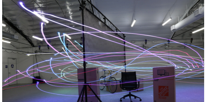
Fig. 1. Long exposure of 32 Crazyflie nano-quadrotors flying through an obstacle-rich environment.
